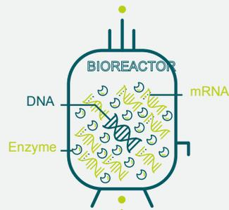
To manufacture mRNA at a large scale, we use biochemical reactions, similar to those occurring in every cell of the human body. This reaction can be replicated with a bioreactor in a so called in-vitro transcription (IVT). This enzyme-based process "translates" a DNA template into mRNA. Due to the highly specific and effective enzyme RNA polymerase, more than 500 mRNA copies can be produced with one DNA molecule.
